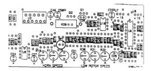
The dynamics and speeds of the KBR-3D's horn motor and low rotor simulator are calibrated at the factory to simulate a 147 type rotary speaker that is well used but maintained. Three parameters of the horn and low rotor simulator may be adjusted to user preference as follows (note original position of potentiometers before turning). The controls for the horn and simulator are labeled:
